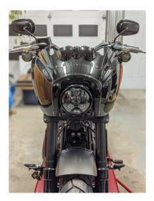
8. Install the pre assembled T-Sport Fairing Billet Windshield Arms (2x) onto the inner fairing brackets using supplied 1/4-20 hex bolt (4x), locknut (4x) & washers (8x). Install in place but leave the arms enough loose so you are still able to play with both arms in order for you to install the windshield more easily. Refer to pictures below.
