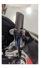
9. Insert larger rubber grommets (2x) inside lower windshield mounting holes & Rubber-Coated Brass Insulating Rivet Nut (2x) inside the fairing shell lower windshield mounting holes. Refer to pictures below.
