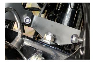
5. Install your fairing shell onto lower and upper fairing mounts using supplied ¼-20 hex bolt (4x), locknut (4x) & washers (8x – one on each side). The fairing shell brackets (Left & right) go on the inside of the upper & lower fairing mounts. Put the nut on, facing the rear of the bike. Also be carefull not hitting your tank with your key/ratchet while you thigh it down. Recommended Torque 15 ft-lbs.
