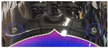
10. Using some blue threadlocker, pre install through your windshield the upper windshield hardware so it hold onto the screen with the supplied rubber washers in the back of the shield. Refer to pictures below (next page).
