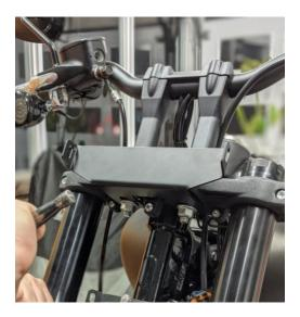
4. Install the supplied headlight bracket kit under your lower triple tree & your lower fairing bracket on top of it according to pictures below using supplied hardware. Lock it down tight by hand. Refer to picture below.
