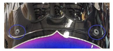
Using some blue threadlocker, pre install through your windshield the upper windshield hardware so it hold onto the screen with the supplied rubber washers in the back of the shield. Refer to pictures below.
