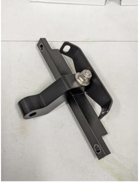
3. Loosen your handlebar risers bolt under upper triple tree until you have enough space to slide under the washer your upper fairing mount.
